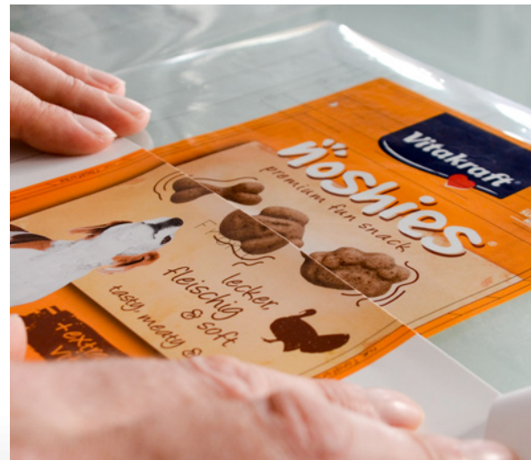
Product images on transparent film and paper proofs are identical in terms of color. (Source: pack.consult)
