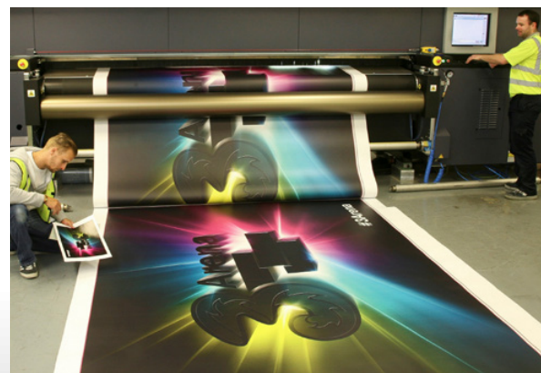
Large Format Print coming out of a digital press (Source: McGowans Print)
