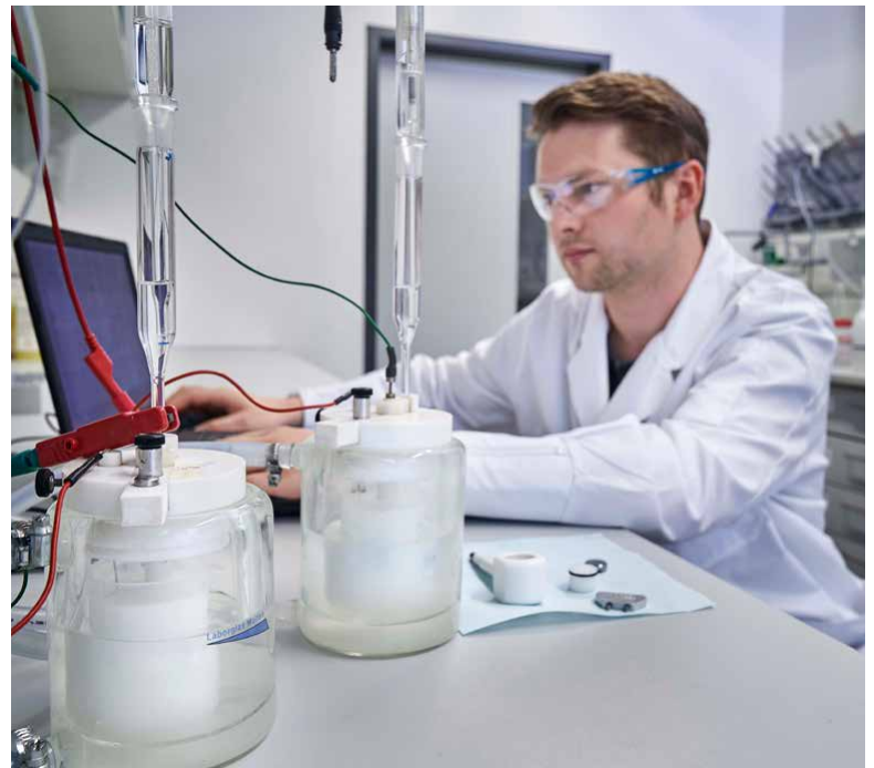
Fogra's release lists ensure that printers don't take any risks with important materials and chemicals. Here in the picture: The testing of dampening solutions.
